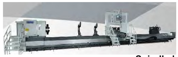
Spindle bore 12" Swing over bed 55" Distance between centers 480"
